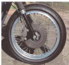
The front 19in Leckford disc brake is from the period and was developed exclusively for the BSA-Triumph works racers and MV Agusta GP bikes.
