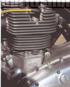
Cylinder barrels used on the racers were warranty returns. Kevlar heat stabiliser, a +10 rebore overcame the necessity of long running-in.
